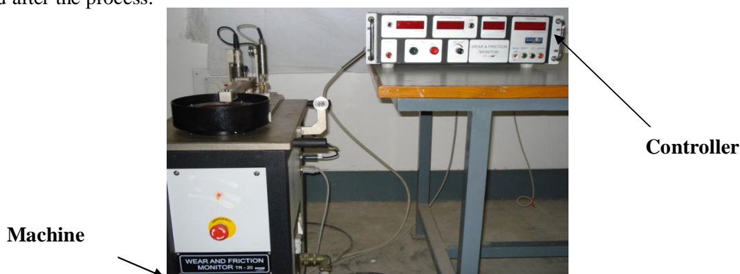
Fig.1 Overall View Of Pin On Disc Apparatus
